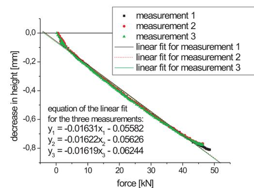
Fig. 4: machine deformation during punch-to-punch compaction
