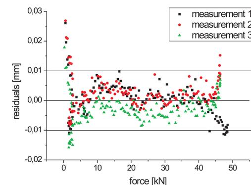
Fig. 5: residuals of polynomial fit 4<sup>th</sup> degree for the data of machine deformation
