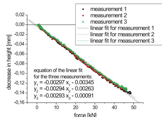
Fig. 3: punch deformation during punch-to-punch compaction
