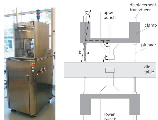
Fig. 1: Stylcam Fig. 2: measurement-setup of the four additional displacement transducers with clamps
