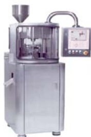
Fig. 1. The Stylcam 100R rotary press simulator
