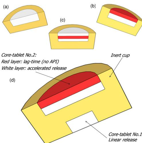
Figure 3. Schematic cross-sections of different types of TIC devices (a) Linear release, (b) Delayed release (lag-time layer in red), (c) Dual-action pulsatile release, (d) End-accelerated release
