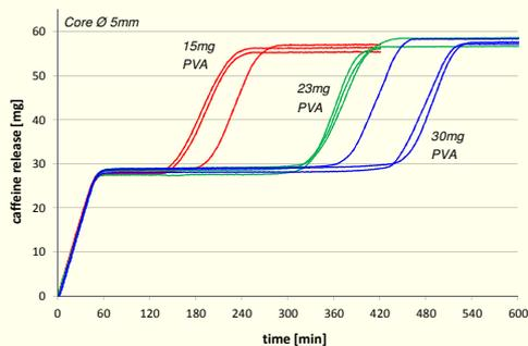
Figure 6. Pulsatile release of TICs with different lag layers (n=3)
