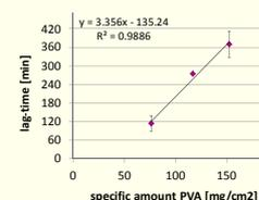
The resulting lag-times had a linear correlation with the specific amount of polymer in the lag-layer (red layer in TIC type (b) of figure 3).
