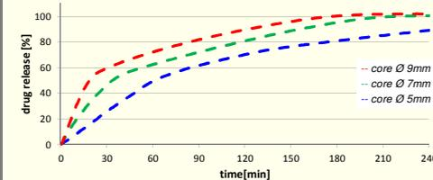
Figure 9. Duloxetine release from TIC type (a) with different sizes
