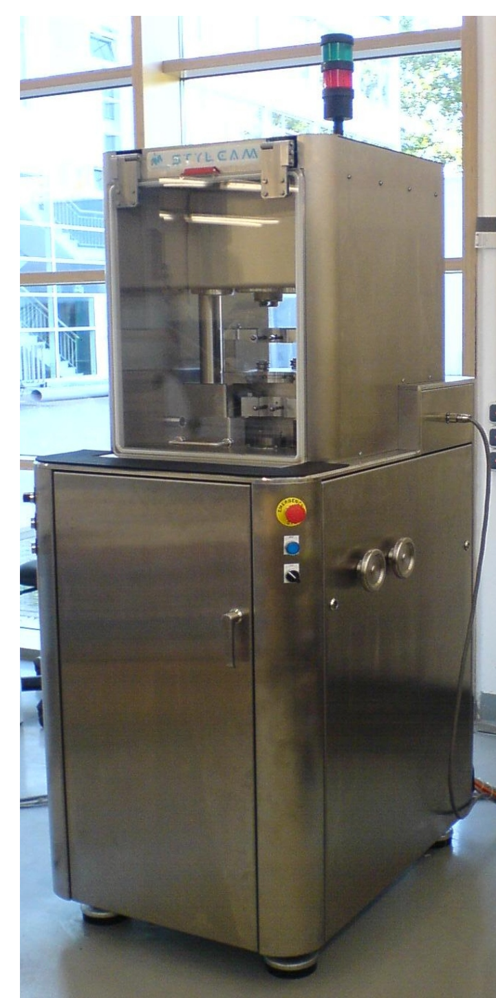
Fig.1: The compaction simulator Stylcam 200R
